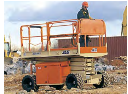
Standard Cross Corner Four-Wheel Drive for Terrainability
