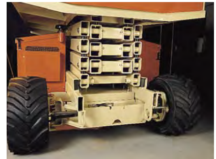
Strengthened Arm Stack for Improved Stack Rigidity
