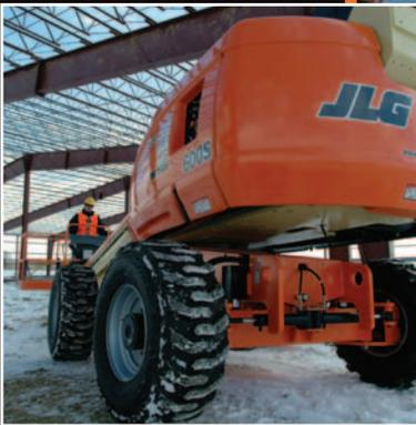
*Oscillating Axle For Improved Traction & Drive Performance*
